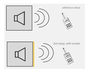
By calculating the difference in sound pressure level between the two setups (one with and one without fabric sample) we get a clear idea of the sound transparency of a material.
