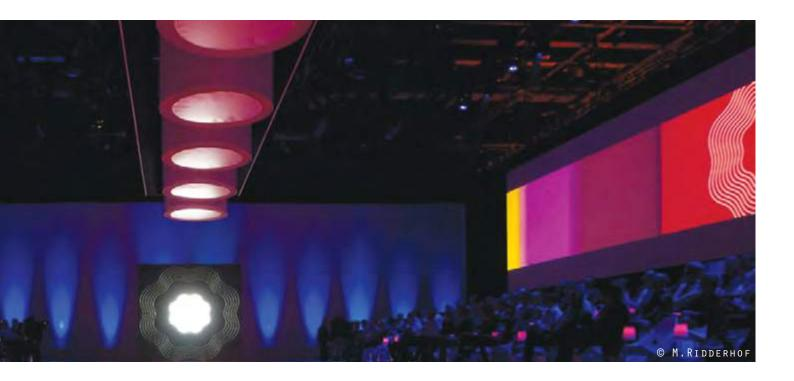
Soft edge blending is a method whereby two or more projectors are used together. The edges of each of the projected images are overlapping, creating a wider display more suitable for showing wide screen content. Obviously, this works best with screens that have a flat gain ratio and therefor reducing the "hot spot" effect and enlarge the viewing area.
