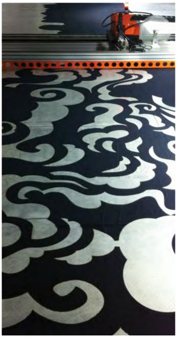
LASER-CUTTING MACHINE CUTTING A BLACK MOLTON CS
